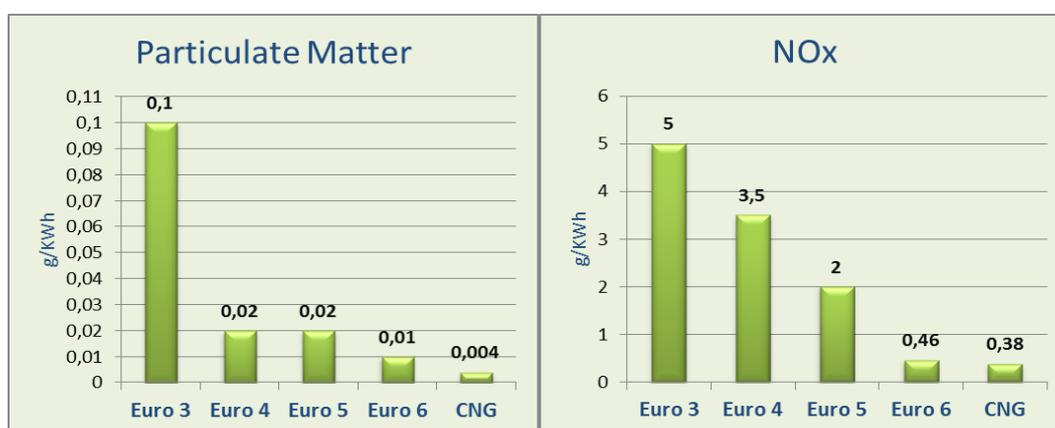
Figure: Assessment of CNG for particulate matter and NO<sub>x</sub> emissions for heavy-duty vehicles. Source: Natural & bio Gas Vehicle Association.
